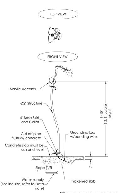
\*\*Not for Construction\*\* Use 4" flange concrete detail
