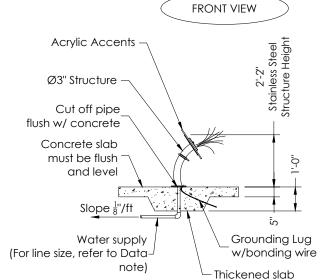
\*\*Not for Construction\*\* Dimensions are given for stainless steel structure. Acrylic accents may add to overall height
